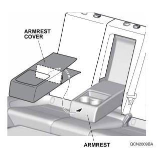
12. Raise the armrest. Pull out the armrest cover between the armrest and left rear seat-back, and secure the fasteners on the armrest cover as shown.
