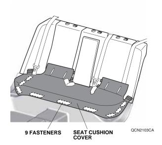
17. Insert the seat cushion cover between the rear seat-back and rear seat cushion.
