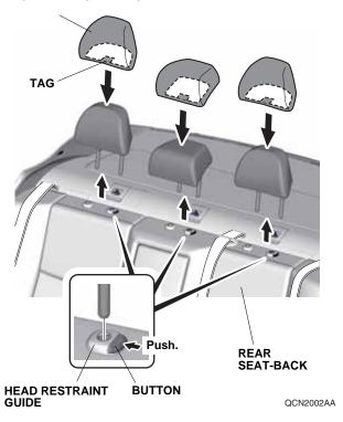
2. Fit the three head restraints covers over the head restraints.
