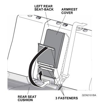
13. Insert the armrest cover between the left rear seat-back and the rear seat cushion. Secure the fastener to the rear seat-back.
