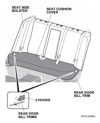
19. Pull the lever, and fold both rear seat-backs forward.
