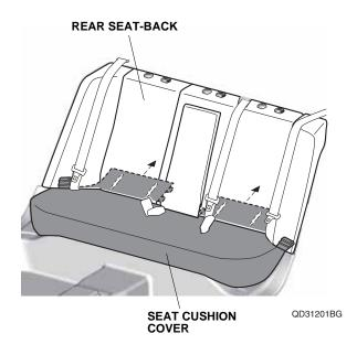
18. Secure the two hooks to the rear door sill trims.
